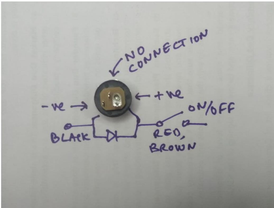
The 1N4007 has to be installed with reverse polarity. Its purpose is to conduct if you have supplied reverse voltage to the radio and burn itself out instead of the radio.
