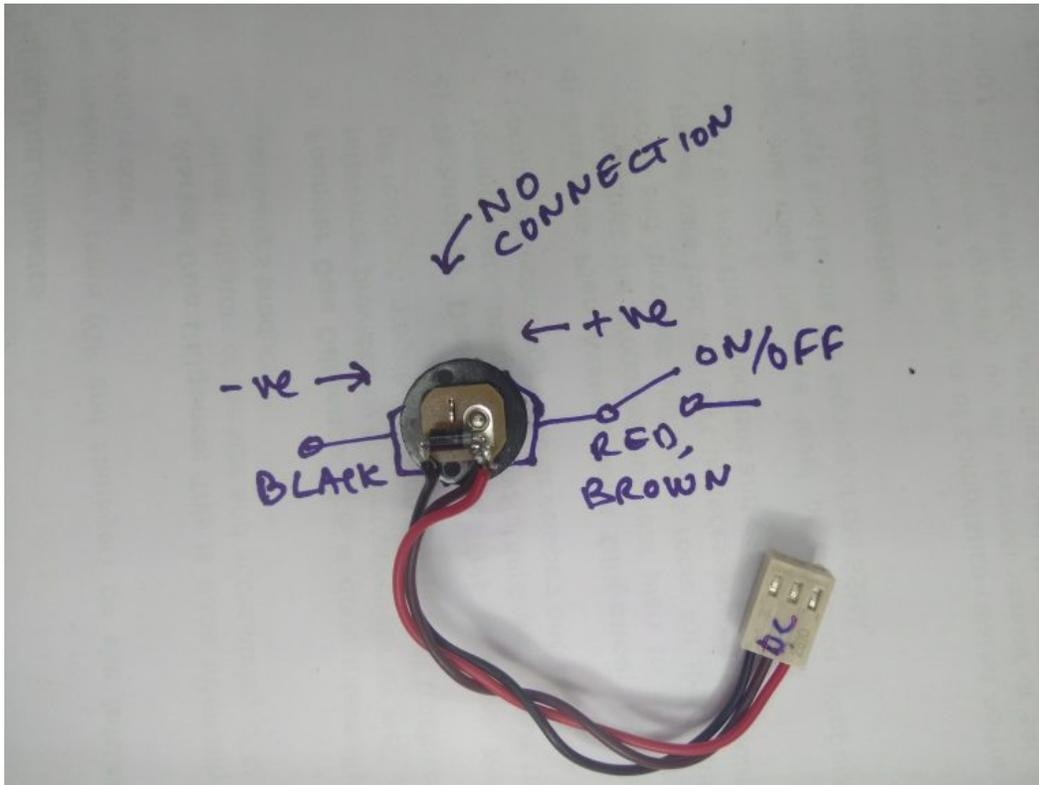
Now, plug this into the main board's DC connector. Switch on the power and measure the current. It should be between 90ma and 110 ma.
