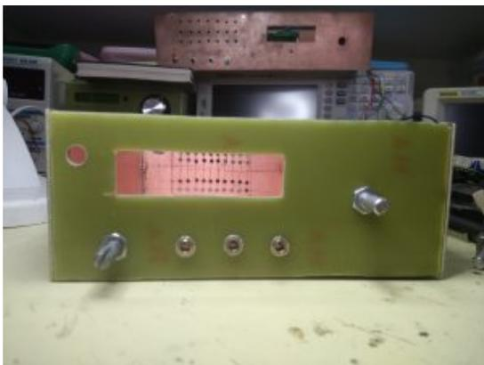
*The front panel controls are installed.*
