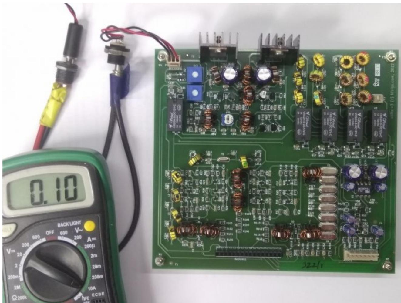
**TIP:** Connect DC connector's ground tab to chassis with a thick wire. The thick wire is needed as a low impedance connection to the chassis prevents ground loops. This applies only if you are using a metal chassis (highly recommended).
